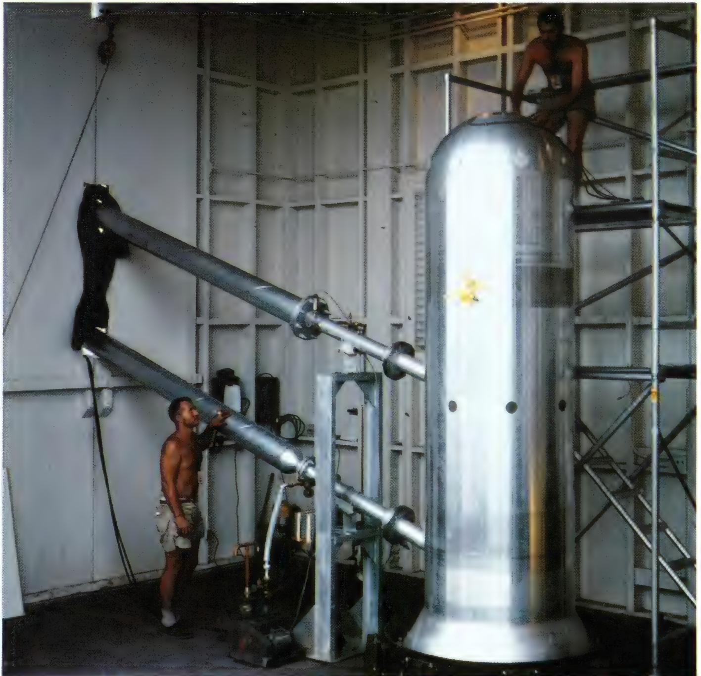
FIGURE 7-33. TEWA DEVICE (D-3, HOB = 8 2' ABOVE WATERLINE)
